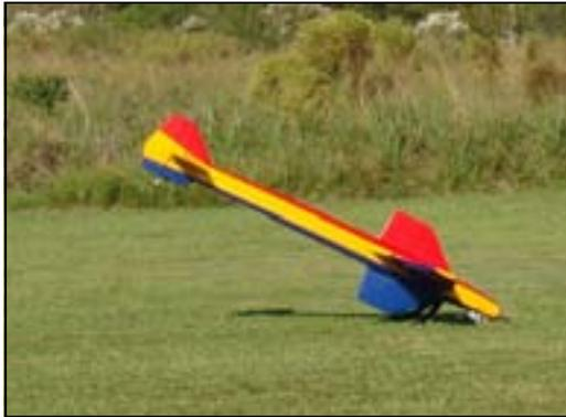
The first picture sure looks like a dart! Initially I had problems landing with the sweep back gear and small wheels. I fixed that with larger wheels that will support the weight of the plane better.
