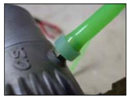
This works great, and it provides about twice the security as tubing without anything. That is, you can pull it off, but you will have to pull twice as hard as you would with just the tubing alone. This should provide more than enough security for most applications. After it has been on/off a number of times, simply replace it with a new piece to restore the original holding force.
