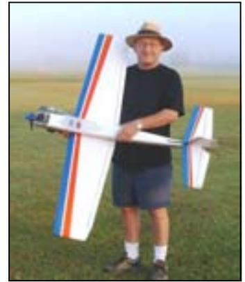
I had originally powered it with a Magnum .52 2-stroke. That lasted only about 10 flights and I was really unhappy about continually adjusting it to make it run. So I took it off and replaced it with an OS .50 SX. Now that is a HOT engine. Puts out 1.8 hp and I originally had a 12x8 prop on it...bad idea with that engine. I had to put a 12x4 prop on it so it would slow down enough to land...used to have to start the approach somewhere in Montgomery County at idle just to get it down.
