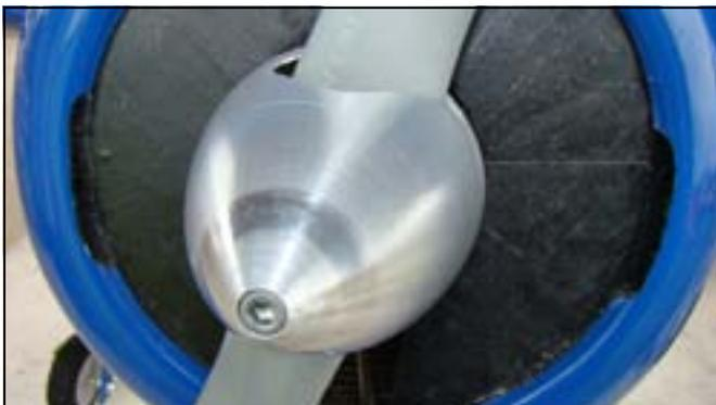
of the cowl I installed a big baffle in the front of the radial cowl to prevent large volumes of air from entering the cowl and becoming static. As you can see in the pictures our club secretary took of the front of the plane, I only made an opening in the baffle directly in front of the engine cylinder.
