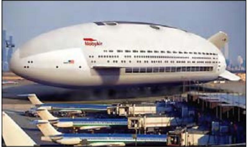
( On a pressurized plane, windows like these would explode outward the Aeroscraft would not fly high enough to need pressurization )
