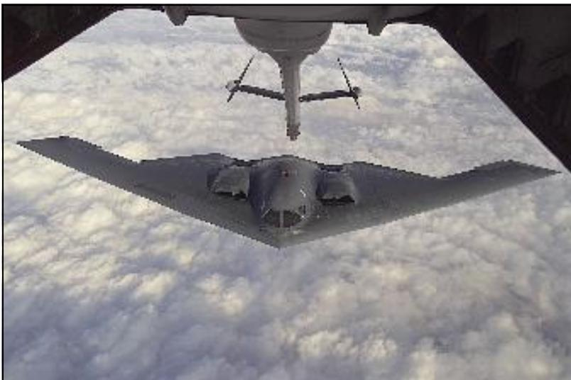
*to detect, track and engage the B-2. Many aspects of the low-observability process remain classified; however, the B-2's composite materials, special coatings and flying-wing design all contribute to its "stealthiness."*
