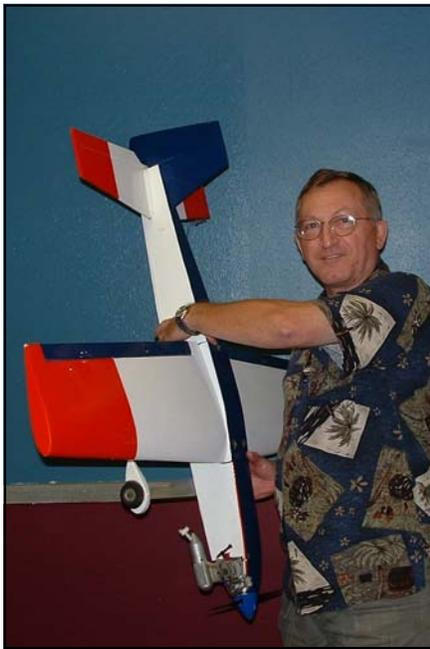
I installed standard 45 oz-in servos for all control surfaces. On the aileron servos, I ran one to the aileron plug and the other to Auxiliary 1 on the receiver. With this hook-up I have both ailerons and they also function as flaps while maintaining aileron function at the same time. I installed a mini HS-81 MG in the fuse due to space restrictions to run the throttle.
