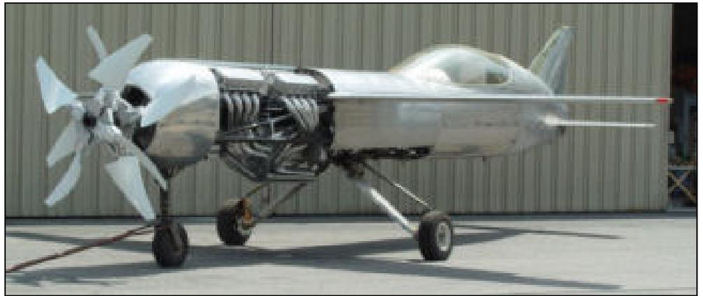
**ENGINES:** Two high performance V-8 engines power the RP-4, representing the best compromise among size, weight, power and availability. Tandem mounted, each engine drives its own propeller. The front engine drives the front prop directly and the rear engine, through gearboxes which bypass the front engine, drives the rear prop in contra rotation. Independent fuel and cooling systems allow for single engine operation
