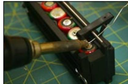
*Many people damage their battery packs before they use them for the first time with poor soldering techniques. Remember to use an iron with a large enough tip to transfer heat, apply solder to the items being joined and not the iron itself, and don't hold the iron onto the battery for too long.*
