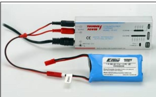
*Many LiPo batteries come with safe charging circuitry integrated into it. This circuitry prevents over charging, over discharging, and in some instances helps to balance the pack out. If your pack has a "Charge" lead on it, always charge through that connector*
