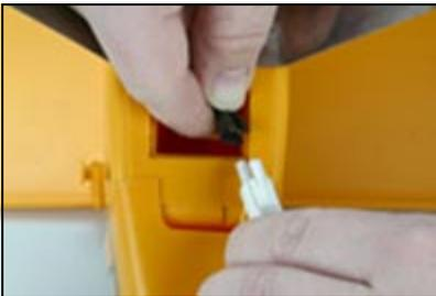
*While a battery may be a battery in many instances, the connectors can vary quite a bit. This battery from a HobbyZone Firebird Commander 2 is similar in dimensions to the standard ParkZone J3 Cub's pack, but the connector is significantly different*
