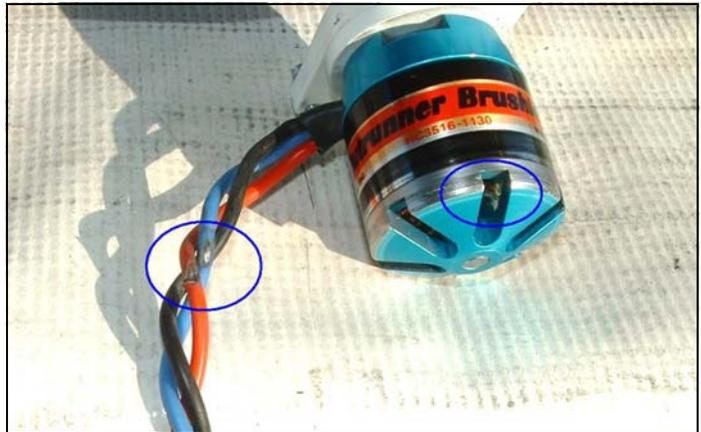
The symptoms of this were strange. I would be flying along fine and without warning, the motor would make an odd sound and it would cut off and on momentarily and randomly. When I removed the motor, it worked fine (no shorting then). When I inspected it closer, I saw gray dust in the spinner and knew something was rubbing. That's when I spotted the wires. Fortunately, my CC Phoenix didn't get damaged.
