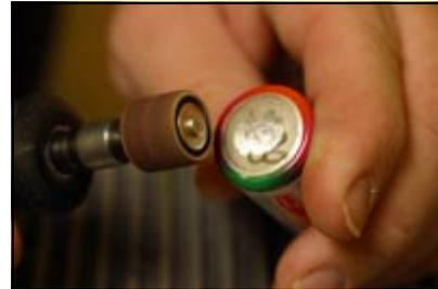
*Some people prefer to assemble their own battery packs rather than buy preassembled packs. Before you solder on the cells, scuff up the terminals to provide a better connection and more secure solder joint.*
