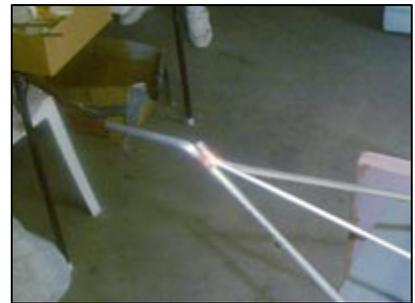
For this demonstration, I am soldering the Main Landing Gear on a 1/4 scale Piper Cub. The Plans require you to solder three wires together into a bundle. The first step is the same as before - Clean all 3 wires with sandpaper. Once they are clean, I wrapped all three together with soft copper wire, keeping the winds neatly aligned .
