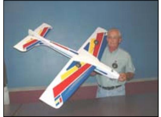
I was searching on EBay one night and did a search for Bridi. I saw the Dirty Birdy for sale and joined the bidding process. The kit arrived in about a week and I started building it. The fuselage is built upside down on the board with a line drawn down the center to make sure the formers are correctly placed. The fuel tank was purchased and installed during the process and is a Hayes 16 oz. slim P/N 146/M.S.R.P.. Construction with triangle stock results in a nicely rounded fuselage.
