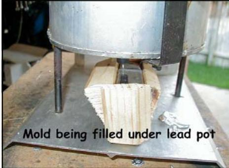
For my pot that's just over 2 inches. You can see what the mold looks like filled to capacity. This is way too much for my needs but the mold will hold a rather large chunk of lead and of course you can make larger or smaller as well as different shapes of molds—whatever is needed for your particular plane.
