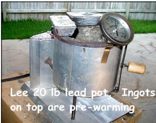
My biggest challenge is that I can't keep the pot full enough when casting. My Lee molds are 6-gang, they cast 6 bullets at a time, and when you are casting six 165 grain ones followed by six 200 grain (.38 Sp and .45 Colt) you run out of lead if you cast too fast (a pound equals 7000 grains for you that are taking notes).
