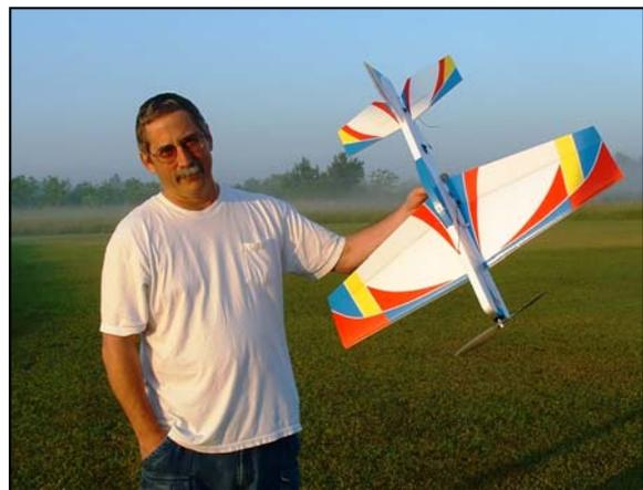
**Photo right**-Bill Murad with his GP Yak 55, 3-D... with a wingspan of 33.5", length, 33", the flying weight is 13.6 ounces. Powered by a Himax 4100 series with 3 Hitec 55 servos and a Castle Creations 10amp ESC, he uses a 3 cell Lithium Ion battery. Back up power, a GE handheld nuclear powered microwave generator. No landing gear is necessary, as the back up power will last for 10 years. I am reluctant to the back up power, as it tends to melt the aircraft....
