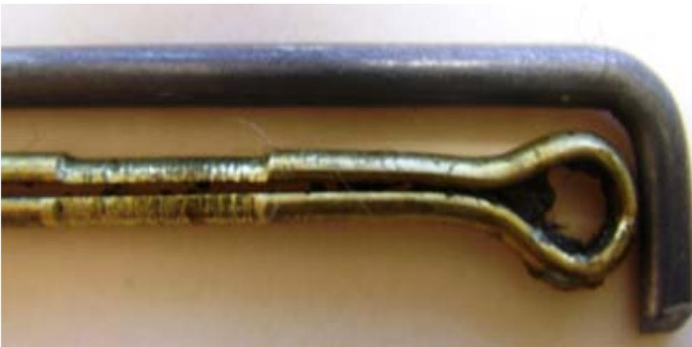
I replaced the standard hinge pins with piano wire. The bend at the end of the new hinge pin is to poke into the balsa, which will stop it falling out, hopefully!!
