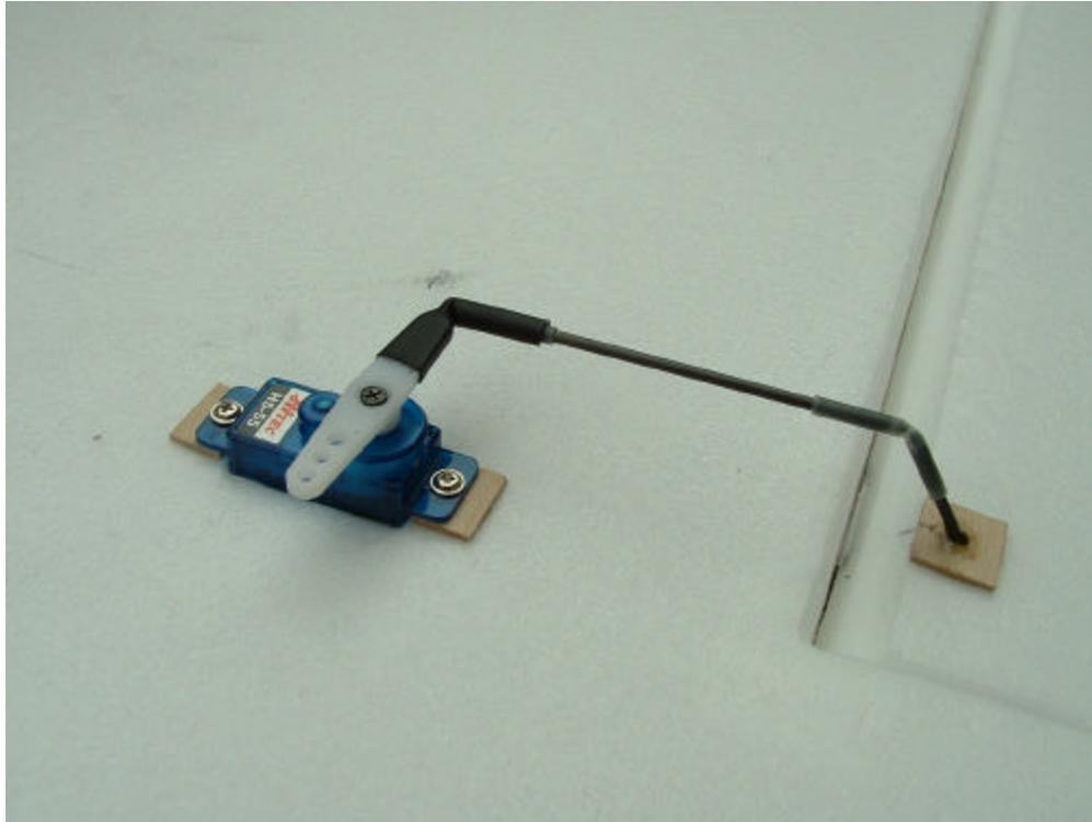
Having recently got into electric flight, where weight is important, take a look at this very light weight pushrod / control horn assembly that I have installed on my Genie. Both the control rod and horn are made from 0.060" carbon fiber rod. The ends of the rod are rounded and connected together with heat-shrink tubing.
