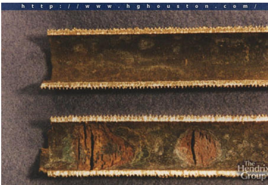
This phenomena is known as 'Stress Corrosion Cracking' or 'Hydrogen Embrittlement'.
